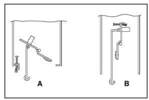
Figure 2 - Damper Operation
